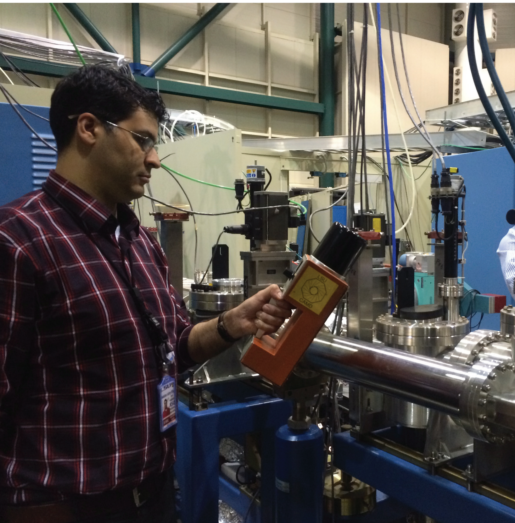
RSO radiation specialist Amin Hamideh (left) and technical assistant Charles Wilson measure the radiation level of the tomography beamline at the LSU J. Bennett Johnston, Sr., Center for Advanced Microstructures and Devices.
