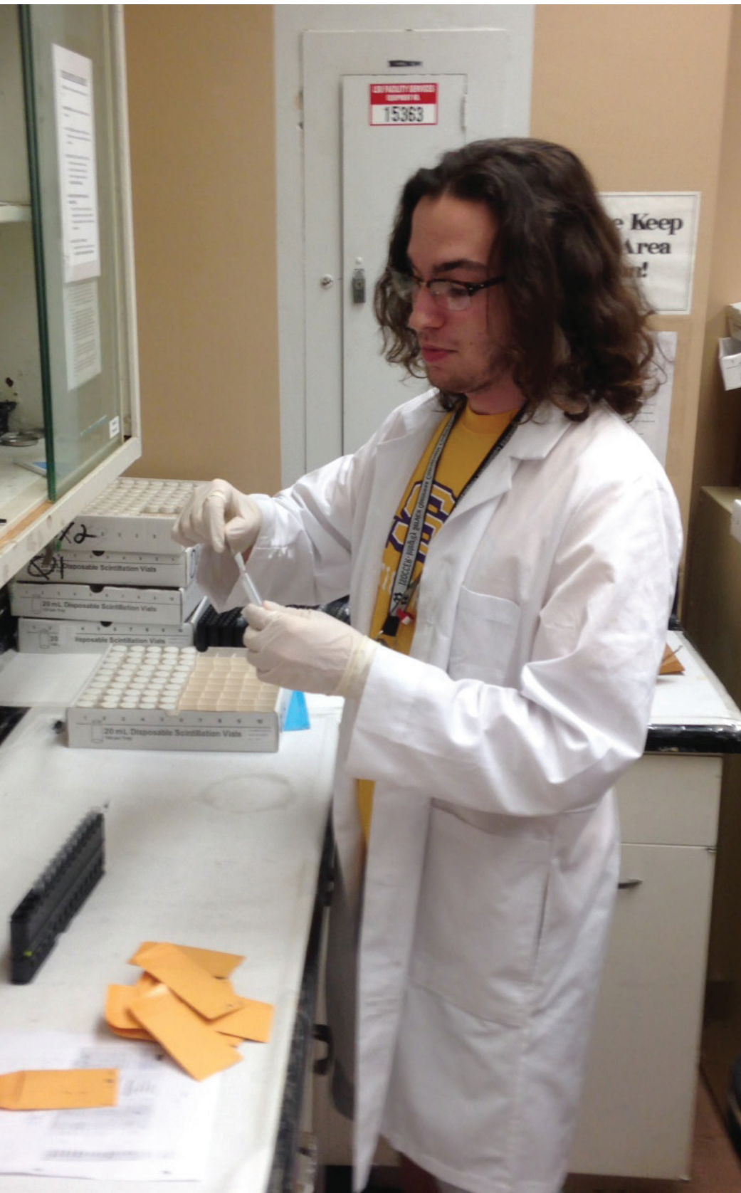
RSO technical assistant Daniel DiMarco prepares smears from the routine radiation laboratory contamination surveys for analysis using a gamma counter.
